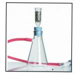
Vacuum filtration. Kit for a quick degasification of samples before analysis.
