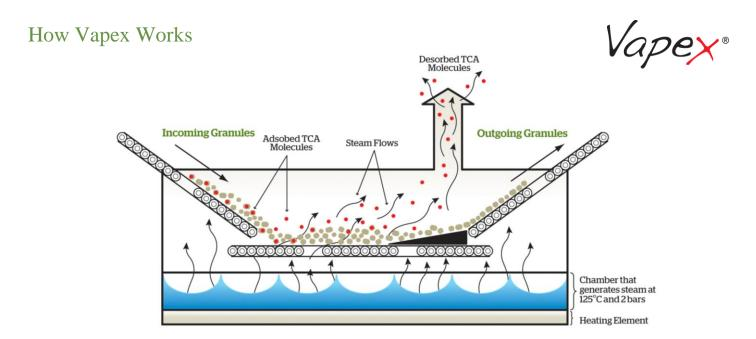
Raw quality-grade cork granules enter a pressurized system through which temperature-controlled steam is continuously pumped. As the heated water vapor flows through the granules, TCA molecules potentially in the cell structure of the cork granules are displaced by water molecules and distilled, along with excess water vapor throughout vents. In the end, ultra-clean cork granules emerge ready to be made into high-quality technical corks.
