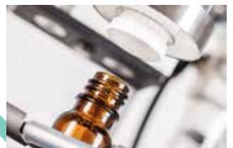
The capping head is powered by a modular pneumatic vane motor with a mechanical compensation system, ensuring proper torque application without damaging either the cap or the container.
