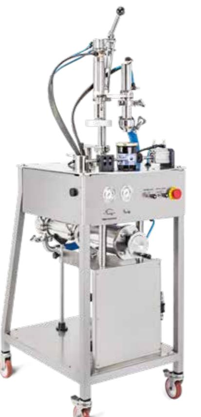
Also suitable for hot filling, it can handle products up to 100°C, maintaining consistent precision even at high temperatures. The pneumatic motor enables capping with adjustable torque, ensuring a secure closure of Twist-Off caps without compromising the integrity of the jar. Adjustments allow control over the force applied to the cap, ensuring a uniform seal.
